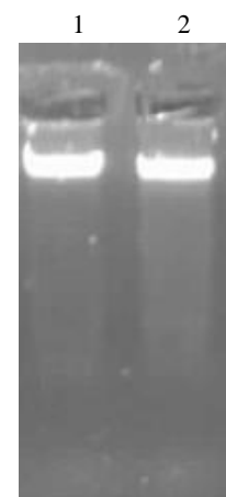
Fig. 1. Agarose gel electrophoresis (1%) for extracted DNA. Lanes 1 and 2 show extracted DNA by optimized protocol.
